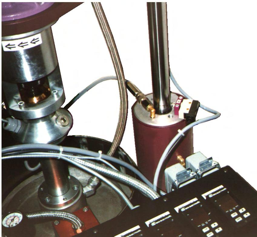
=< End limit switch for the barrel empty control.
