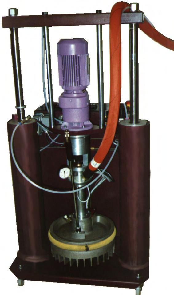
Put the lever of the pneumatic hand valve in the upper position and elevate the follower plate in the upper end position.
